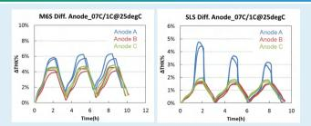
$\otimes$  Two models are used to evaluate the swelling of different anode cells, and the comparison result is almost the same, which is A > C > B
