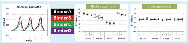
Comparison of the swelling behaviors of four LIBs made by different binders, the level of irreversible swelling is the same, and the main difference lies in the single-cycle swelling thickness, In which the binder-C has the best swelling suppression effect, Thus, it can be used for evaluating And screening different binder materials.
