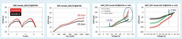
Two types of anode material batteries with the same design and capacity, of which the full charge swelling and irreversible swelling thickness of B are significantly greater than that of A, which can be used to screen and evaluate battery anode materials with swelling requirements;
